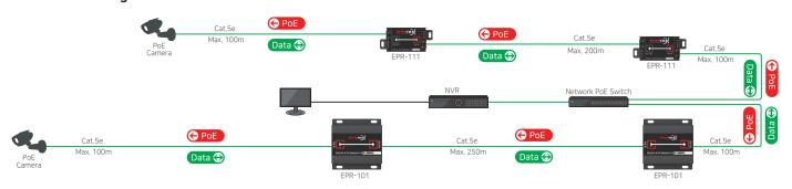
► Transmission distance may vary depending on the type and quality of cable, camera and environmental condition
