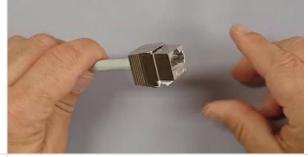
The finished connector should not show any wires at the
