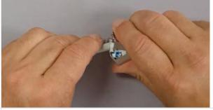
Roll back the braid or drain wire so it will fit under the jack
