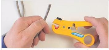
Strip 40mm of sheath from cable using stripper
