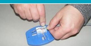
Using working base, place wires as per color spec
