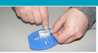
Using working base, place wires as per color spec
