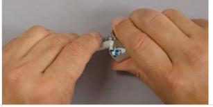
Roll back the braid or drain wire so it will fit under the jack body. Close the rear covers, pressing firmly until the jaws close and click into place
