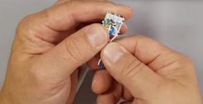
Lay the wires into thier correct configuration, either T568A or Using side cutters, cut the wires level with the wire forming T568B
