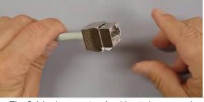
The finished connector should not show any wires at the back, the jacket should reach to the rear of the connector and the braid or drain wire should be tidy underneath the shield bodv.
