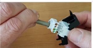
Place the wiring cap into the connector body using the arrows on the cap to match on the body
