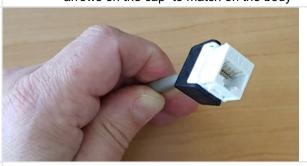
The finished connector should not show any wires at the back, the jacket should reach to the rear of the connector .
