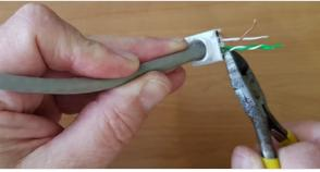
Lay the wires into thier correct configuration, either T568A or Using side cutters, cut the wires level with the wire forming
