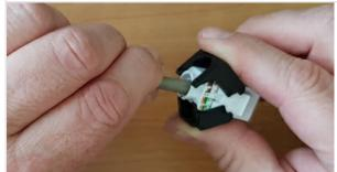
Close the outer clamps around the connector body.
