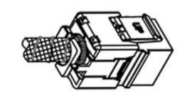
Step 4: Press tool to terminate the jack and cut off the excess Step 5: Place the cap on the jack and press to make sure it is fully seated. Put the hinged side cover into the slot. Snap the side cover to the jack
