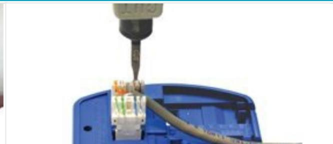
Terminate wires using standard 110 impact tool
