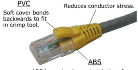
ABS has a harder material, therefor no fall off after crimping.
